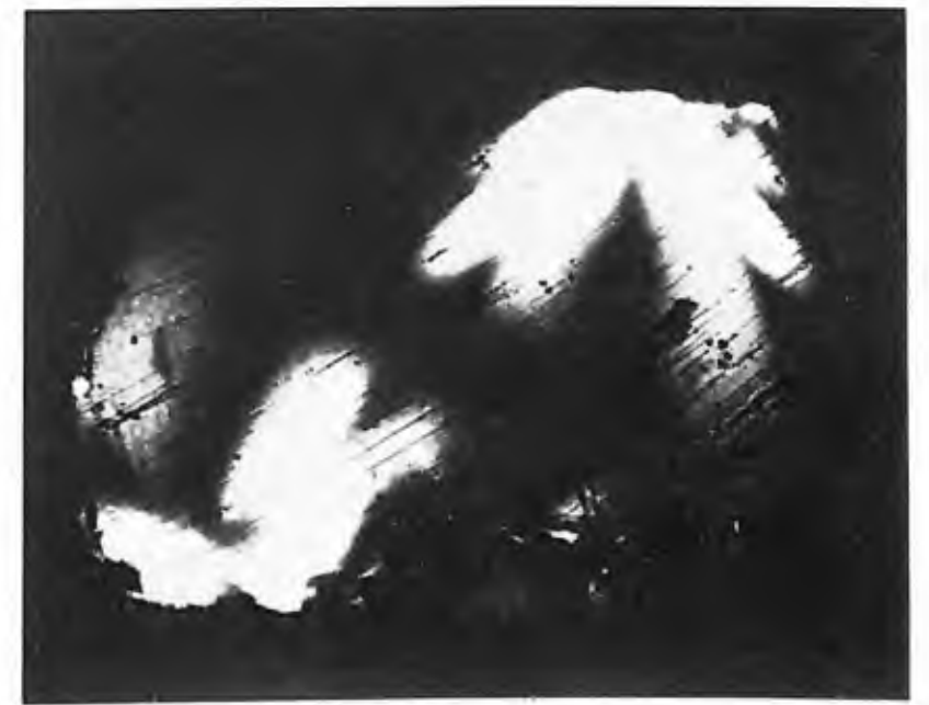
Right: The same lithium fluoride experiment as on the previous page, observed using polarizing light. Regions of high stress are shown with greatest illumination. The striations are spreading out from the lower left-hand corner and the upper right-hand corner of the crystal
