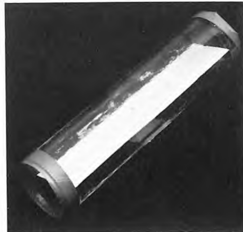
Right: A metal plate in a sealed quartz glass tube covered with a chemical, fluorescing in ultra-violet light Below: Copper rod with wires soldered to it to measure any electrical effects in the rod during bending
